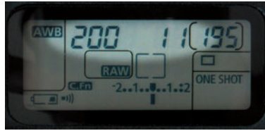
FIGURE 7.45 Here, our camera indicates that it has calculated an exposure of 1/200^{\text{th}} of a second, at f/11 .
